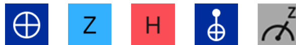
Fig. 9: Symbols for Pauli X (NOT), Pauli Z, Hadamard (H), conditional not (CNOT) and measurement gates used in IBM Q Composer.
